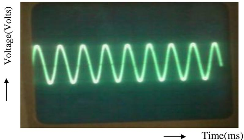
Fig.4.19f. Output Voltage of the Inverter 2
