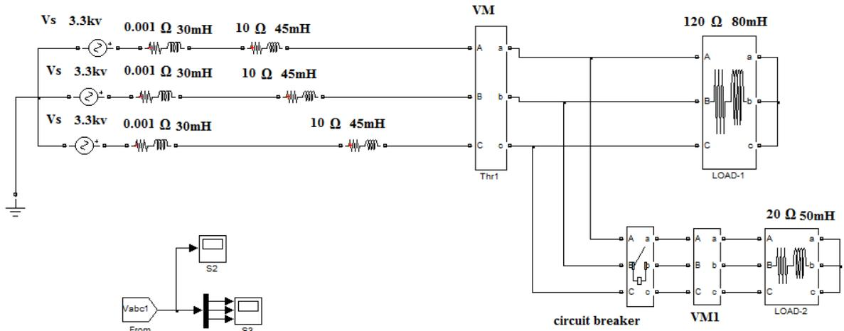
Fig.4.10. Circuit Model of Three Phase System with the additional load
