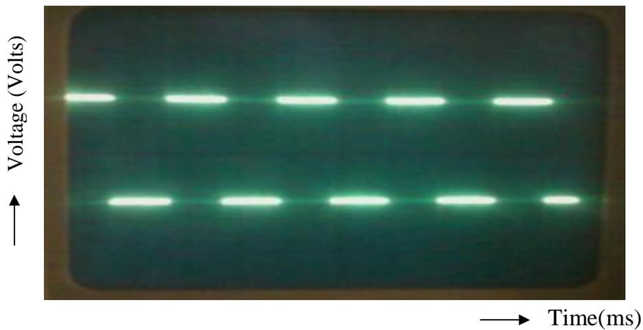
Fig.4.19e. Output Voltage of the Inverter 1
