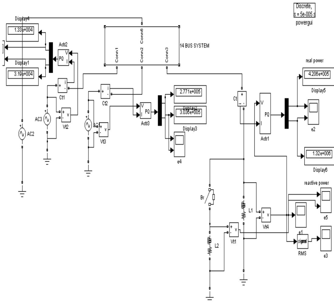
Fig.5.6.1. Fourteen Bus System without UPQC
