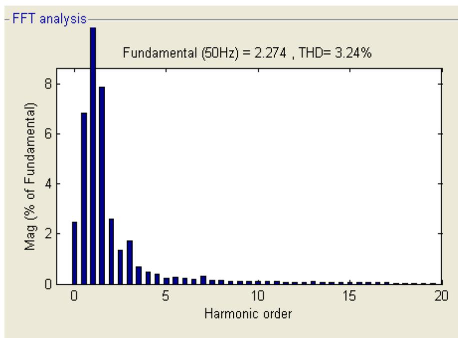
Fig.5.8.2.32. Frequency Spectrum for Current.
