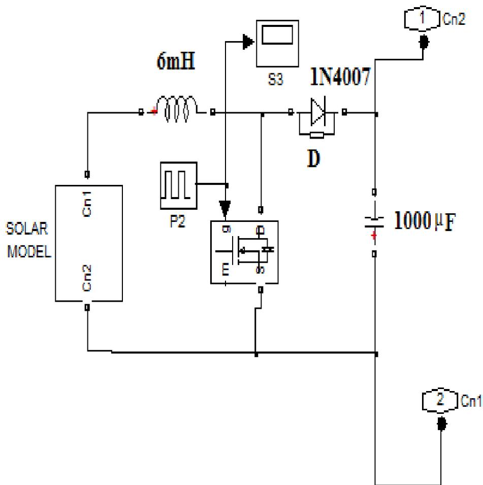
Fig.4.3. Boost Converter Circuit
