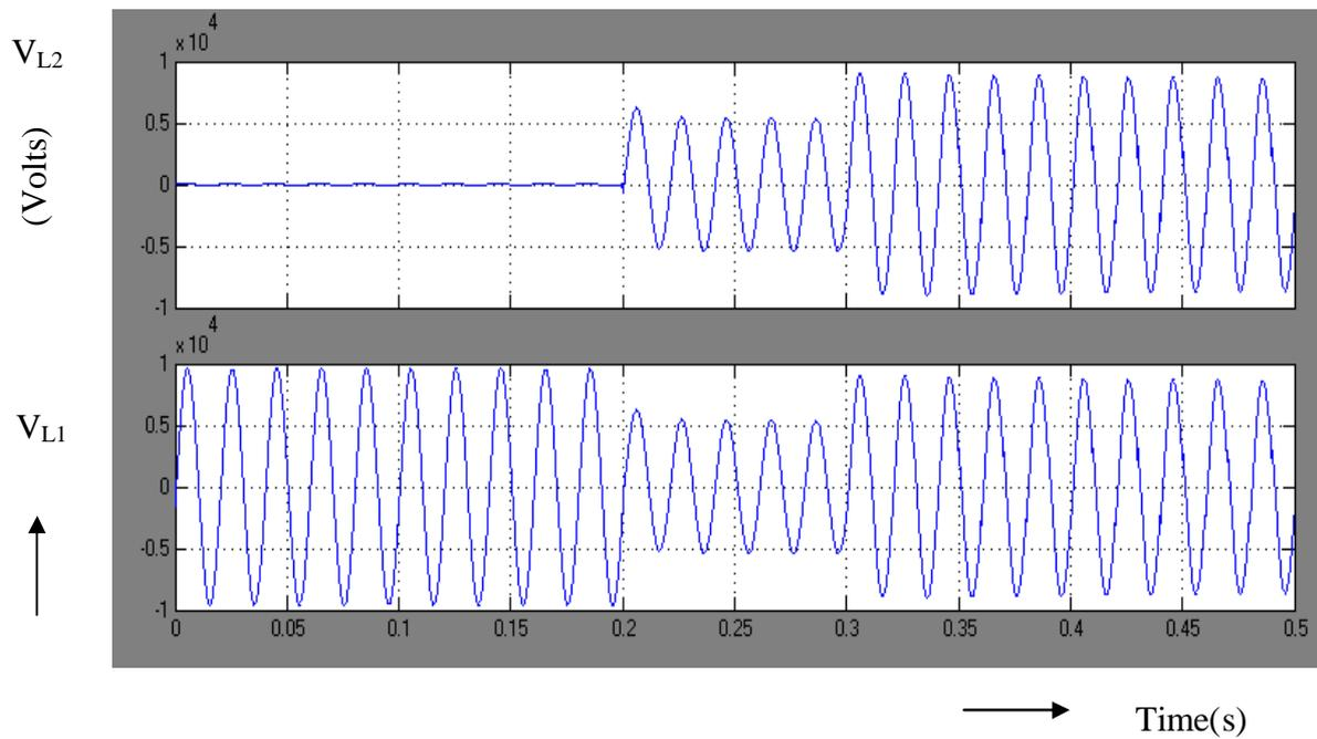
Fig.4.4 Voltages across Load-2 and Load-1
