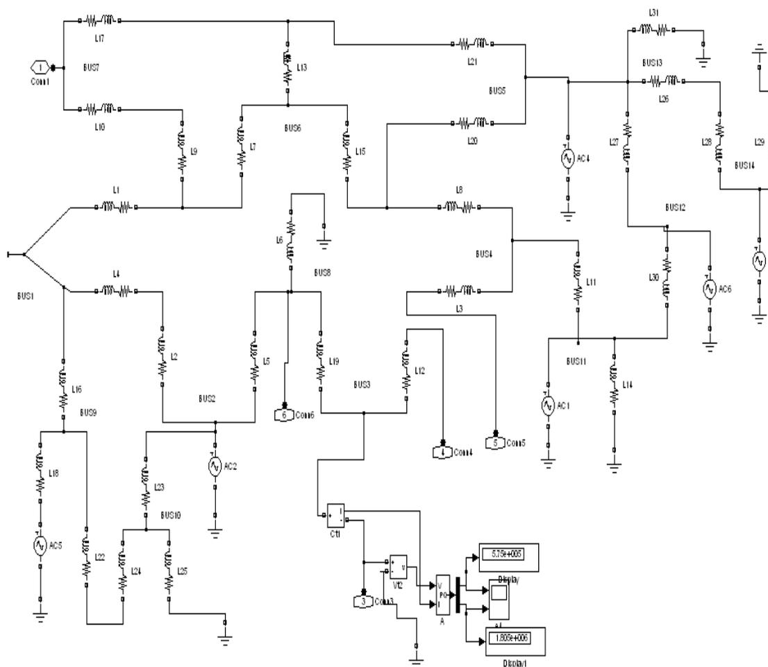
Fig. 5.6.6. Circuit model of 14 Bus System
