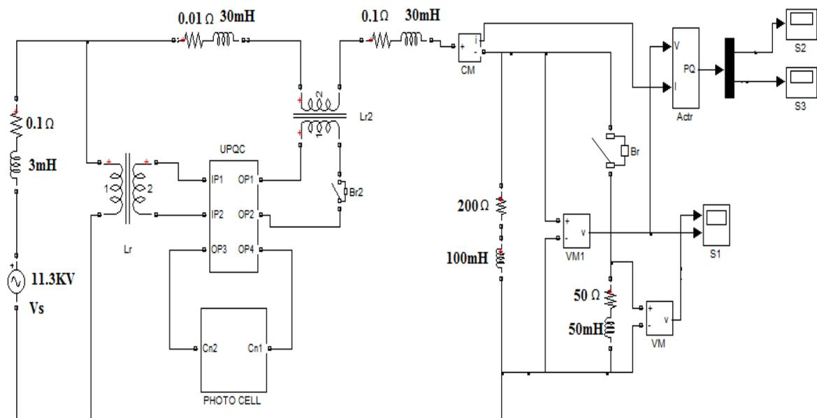
Fig.4.1 Circuit model of the UPQC System
