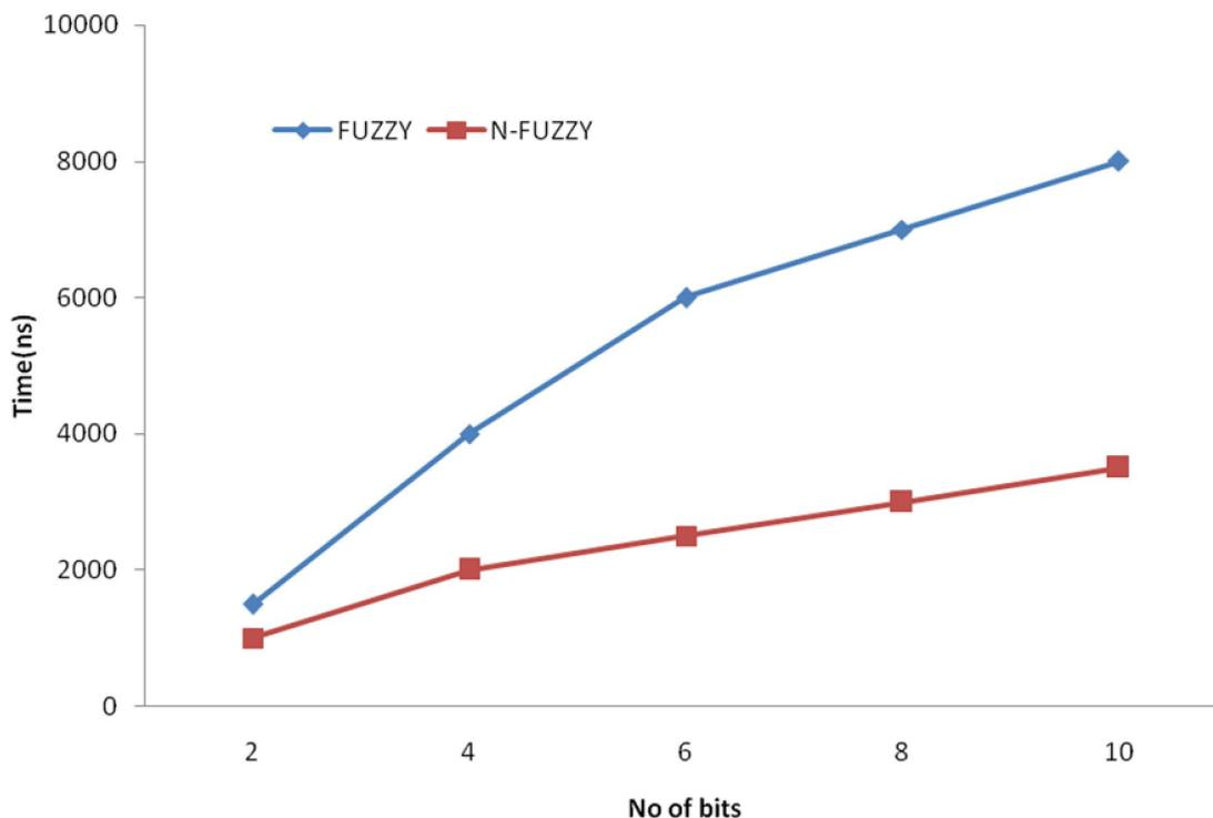
Figure 4.4: Delay Performance of Neuro Fuzzy Logic
