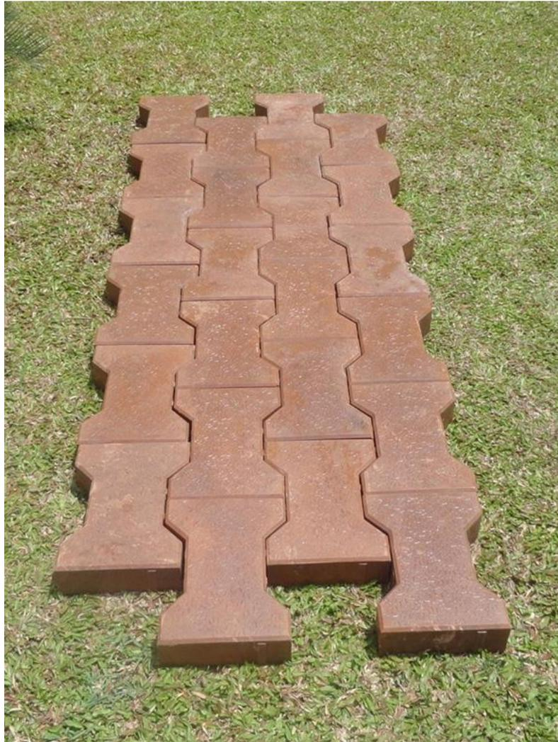
Fig.1 Paving blocks produced from fly ash red mud combination. (Anuj Kumar et al.)
