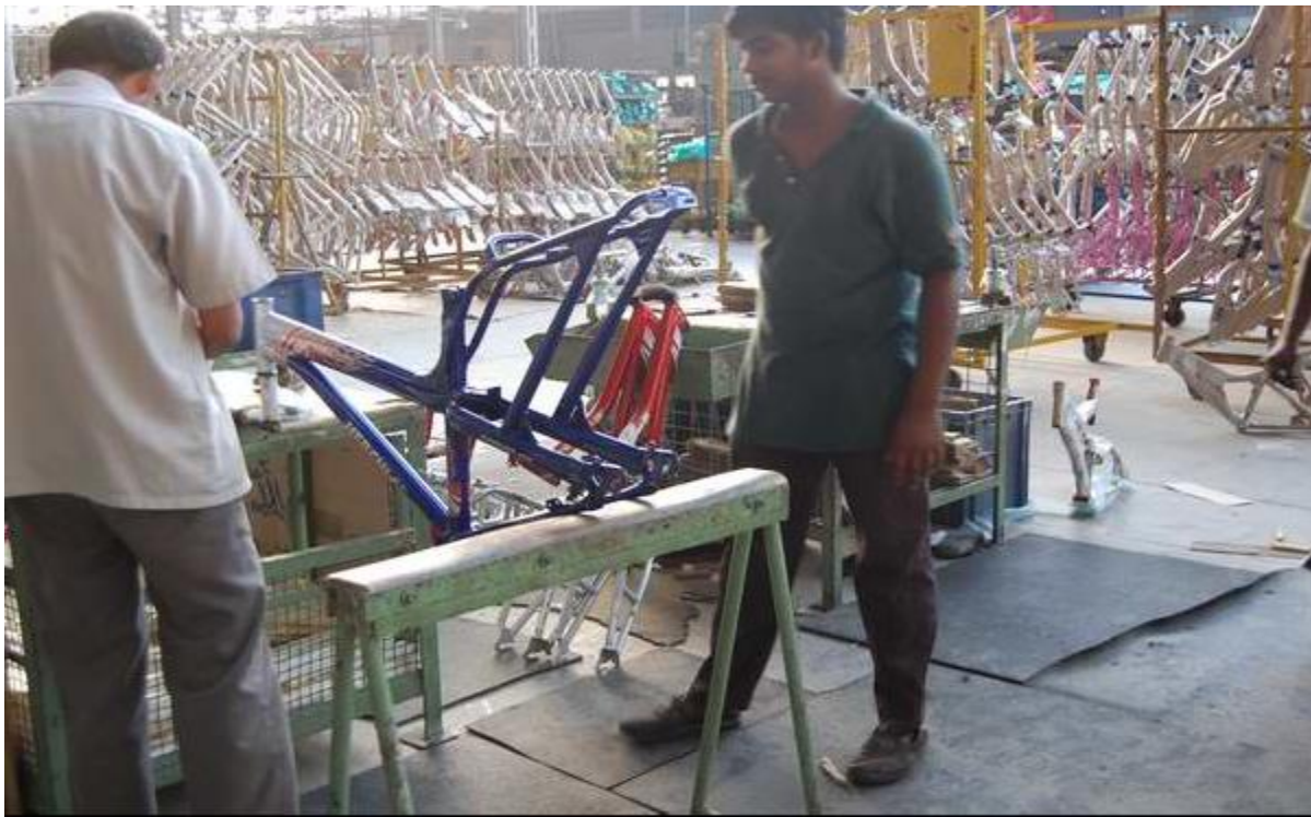
Decorating works on the frame
